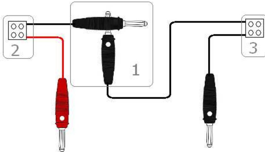
Now we measure electric current in the circuit between the red and black plugs. We can connect the voltage source (a solar panel) to one connection (2) and the voltage consumer to the other (3) connection.
