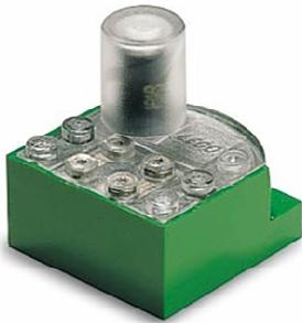
The capacitor has a capacity of 1 Farad and is protected against an excessive voltage of 18 Volts. Completely charged up to 2,5 Volt it will contain 3,125 Joules. The LEGO brick also contains a LED which will start blinking when the capacitor is fully charged.
