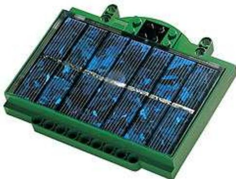
The solar panel consists of seven solar cells and one diode. The solar cells are connected in series. The solar panel will have a maximum voltage of  $7 \times 0,4$  V. In full sunlight the solar panel will produce 100 mA indoors and 200 mA outdoors. Using 60 W lamp at a distance of 25 cm the solar panel will produce 2,5 V and 8mA. However if we decrease this distance to 8 cm it will produce 2,5 V and 40 mA.
