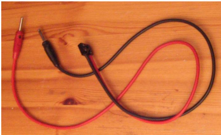
Now we're able to measure voltage by simply putting our LEGO connector on any other LEGO connector. However if we want to measure electric current we'll need two of our self-made wires and we'll have to connect (1) them as seen in the picture below:
